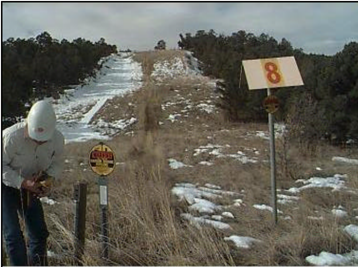
Cathodic protection measurement performed at right-of-way crossing
